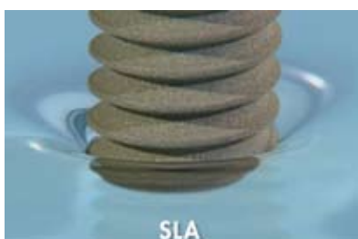
Fig. 3: Immersion of SLA and SLActive implants in water demonstrates the wetting of SLActive and its meniscus at the water-air-implant interface.
