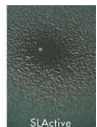
Fig. 4: Demonstration of the superhydrophilic property of SLActive. Note the refractions below the water droplet resulting from air bubbles entrapped between the water and the SLA surface.
